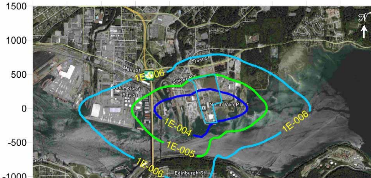
Figure 4 Individual Risk Distribution around the Plant – Potential Future Plant: Operations after Technology Conversion
