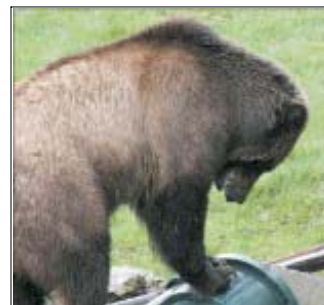
A bear can knock this bin over and jump on it, but still can't get inside it, during testing of three types of garbage bins.
